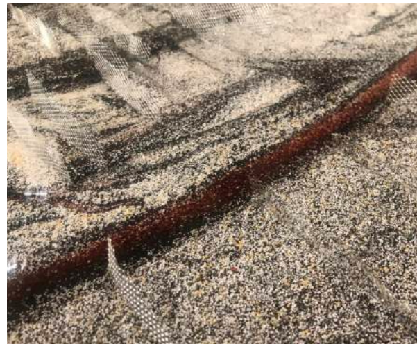
WIRE MESH SIMULATING VEGETATION STABILIZATION
